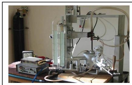
Fig. 5. The 3 kW laboratory scale DC transferred plasma arc reactor
